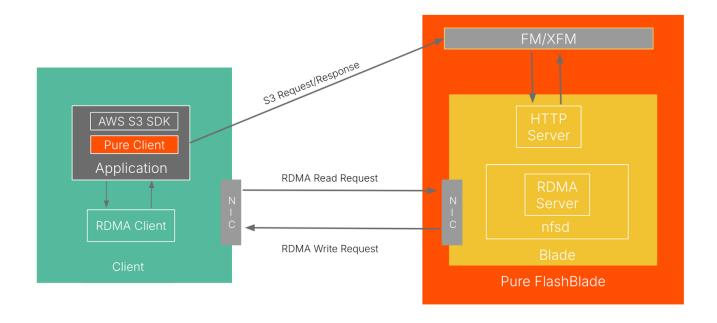
Figure 1. How S3 over RDMA works for FlashBlade.
